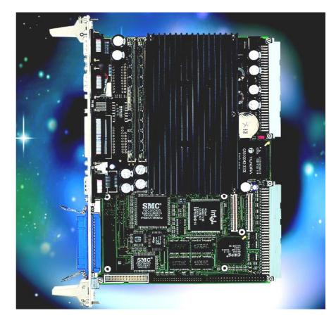
The *VP6* VMEbus all-in-one 6U single board computer is designed to meet the needs of embedded application developers addressing markets like telecommunication (high bandwidth, broadband data or intelligent network switching), industrial automation, military and aerospace, medical, scientific, and imaging. Supported operating systems are Windows NT, Windows 98, MS-DOS, QNX, VxWorks, Solaris and others.
